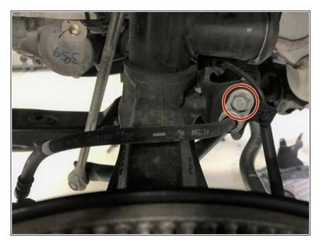
Use a 12mm socket and ratchet to remove the bolt shown with red circle
