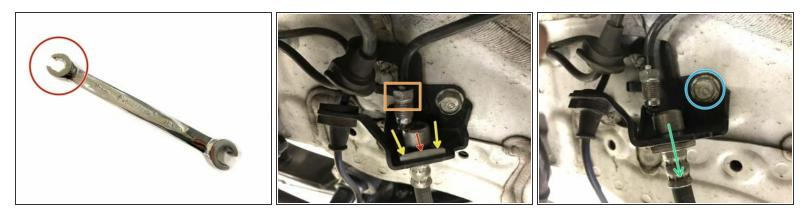
▲ It is critical to use a Line Wrench to loosen the brakeline connection. Using the open end of a standard wrench may round over the corners
