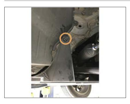
Re-install the push clips at each side of the undertray
