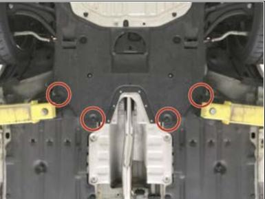
Re-install the 10mm bolts with a 10mm socket & torque wrench. Torque to 8-12 ft-lbs
