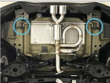
Then raise the rear end of the muffler section up and insert both rearward hangers
