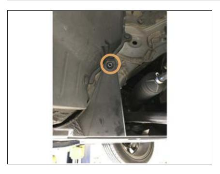
Re-install the push clips at each side of the untertray
