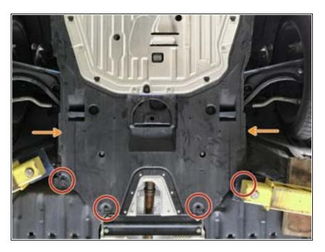
Re-install the 10mm bolts with a 10mm socket & torque wrench.
