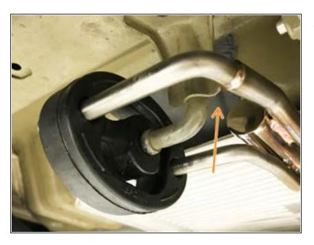
Verify that the hanger bar is not contacting the chassis. Move the muffler section rearward if the hanger bar is very close or touching the chassis
