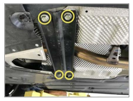
Re-install the cross member. Use a 14mm socket & torque wrench to torque the bolts to 25-35 ft-lbs
