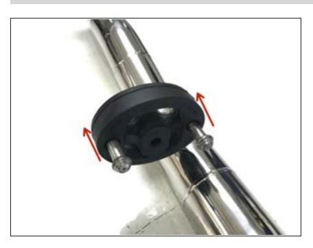
Position the rubber hanger as far forward on the hanger rods as possible to provide clearance for the chassis hanger rod
