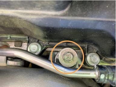
Undo 10 mm bolt on the inlet pipe as shown
