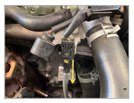
Unplug the lower oxygen sensor electrical pigtail connector located next to the upper oxygen sensor connector
