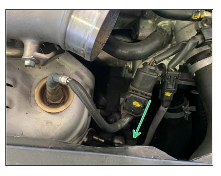
Undo upper oxygen sensor electrical pigtail and let loose out of the way
