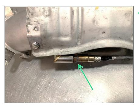
Swap lower oxygen (O2) sensor from OE downpipe to 27WON Downpipe
