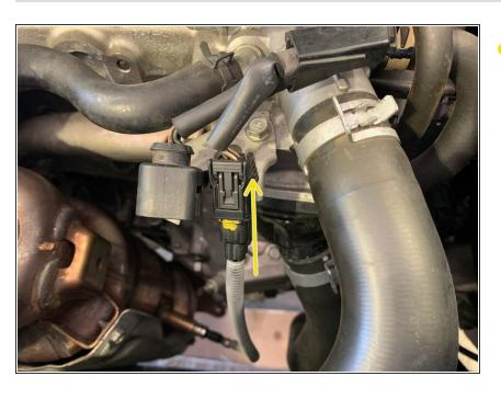
Reconnect the lower oxygen sensor electrical pigtail as shown
