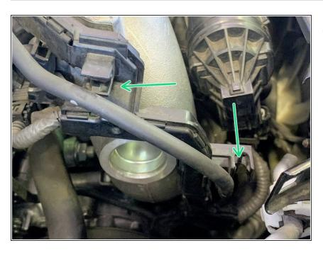
Unclip the vacuum hose from the clips on the vacuum line retainer bracket
