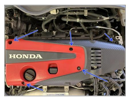
Use a 10mm socket and install the 5 bolts to hold the engine cover
