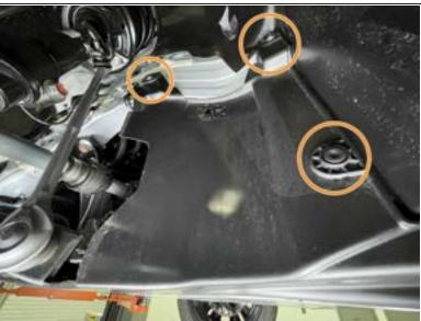
Use a large flat head screw driver or prying tool to remove the four (4) push-clips in each front wheel well
