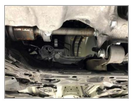
Remove the OE front-pipe from the vehicle through the access point directly under the engine
