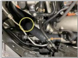
⚠ In this process try not to disrupt the assembly between the hot side pipe and turbo outlet silicone. You want to maintain the alignment
