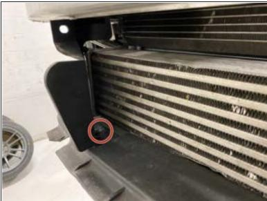
Use a flathead screwdriver to remove the two (2) push clips
