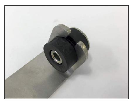
Install the OE rubber mount and steel collar as shown
