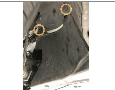
Re-install the push clips at the side of the undertray
