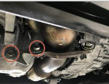
Use a 14mm socket or wrench to install the four (4) 14mm bolts and brackets. Torque to 38-42 ft Ibs
