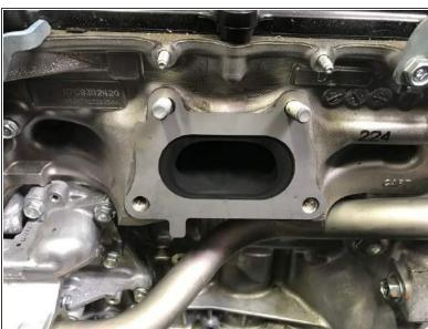
Locate the provided turbine inlet gasket and install as shown
