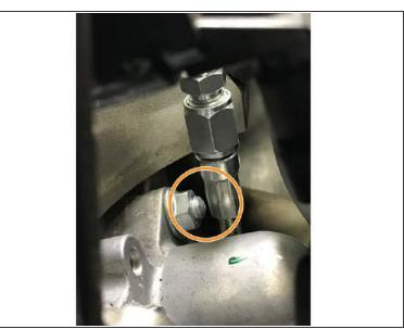
Use a 14mm socket and torque the oil feed banjo bolt to 12-14 ft-lbs
