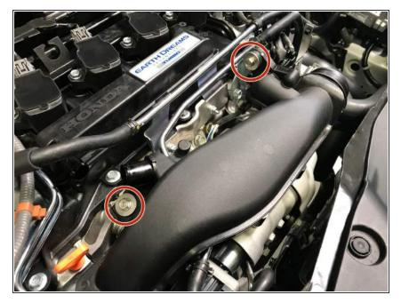
Use a 10mm socket & ratchet to remove the two (2) TIP mounting bolts
