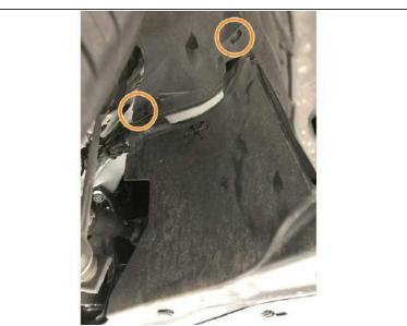
Use large flat head screw driver to remove push-clips on each side of skidtray
