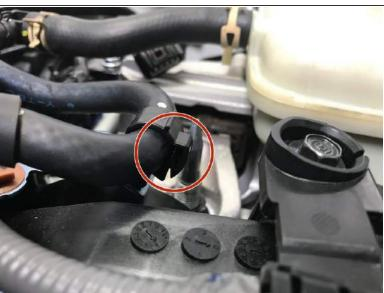
Reinstall the plastic clip holding the upper coolant hard lines and rubber hose
