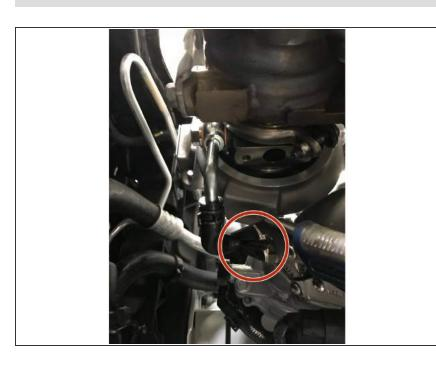
Remove the vise grips from the lower coolant hose
