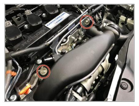
Use a 10mm socket & torque wrench to install the two (2) TIP mounting bolts. Torque to 8-10 ftlbs
