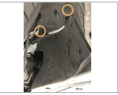
Install the remaning six (6) push-clips on each side of the skidtray
