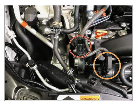
Install the wiring harness back onto the bracket
