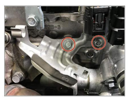
Use a 10mm socket & torque wrench to install the two (2) 10mm bolts and bracket. Torque to 8-10 ftlbs
