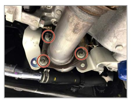
Use a 14mm socket & torque wrench to install the three (3) 14mm nuts/studs. Torque to 30-40 ft-lbs
