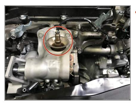
Use the specialty O2 sensor socket to install the primary O2 sensor.
