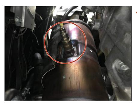
Use the specialty O2 sensor socket to install the secondary O2 sensor.
