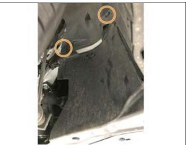
Use large flat head screw driver to remove push-clips on each side of undertray
